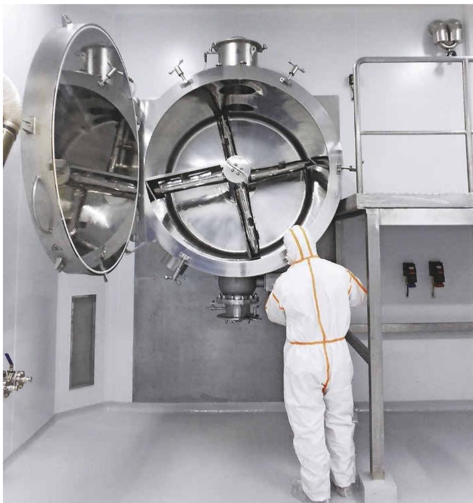
*Internal and external cleaning of the Cosmodry system is very easy. There is no support frame occupying the sterile room, only the drying chamber flanged to the wall.*
