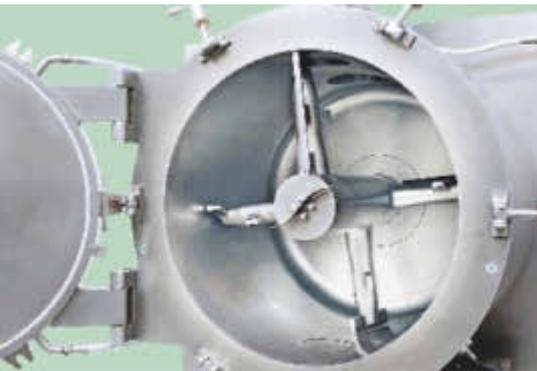
*The agitator can be dismantled into different sections. Its special configuration facilitates heat exchange, thus reducing drying time.*
